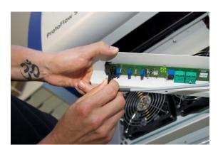
Inserting the "profile recorder" module
